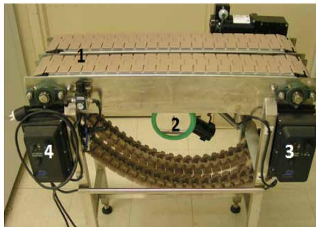
*The prototype trim sampler: divided conveyor, 1; sampling disc, 2; motor fitted for the conveyor, 3; and motor fitted for the sampling disc, 4.*
