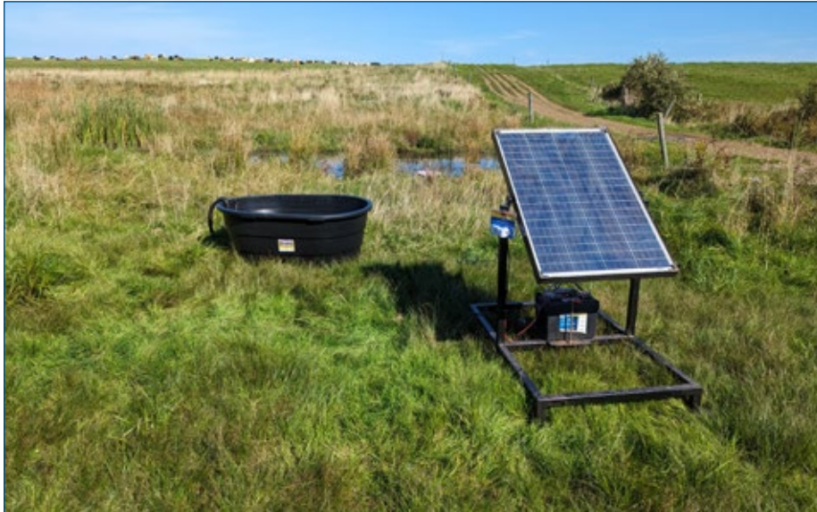
Figure 3.11 A simple setup of a solar panel, batteries and a submersible pump. The pond is barely visible in the background.
