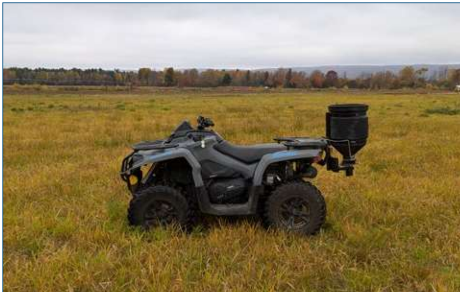
Figure 5.4 Broadcast seeder mounted to an ATV.
