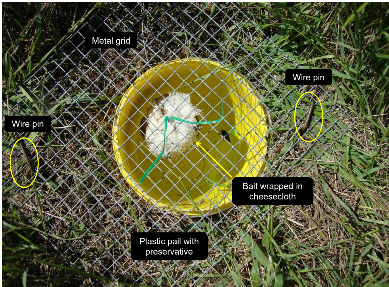
Figure 10. This dung-baited pitfall trap uses two plastic pails (2-litre capacity), one nested inside the other, buried with the lip of the trap level with the soil surface. The inner pail is easily removed to empty trap contents; the outer pail remains in the soil to prevent the hole from collapsing. A wire screen secured with metal pins over the mouth of the trap excludes rodents and birds, and supports a bait made from fresh cattle dung (ca. 250 ml) wrapped in 3-ply cheese cloth and secured with a twist tie. Baits can be made the day of use, or made in advance and frozen until needed. They remain effective for 2–3 days (Bezanson et al. 2020). Preservative (ca. 2 cm depth) in the inside pail drowns and preserves insects attracted to the bait. (Photo: KD Floate).
