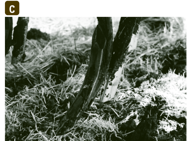
Figure 4.5.3 Four Types of Openers Available to Inject Liquid Manure. (a) Yetter disk opener (b) Sweep opener (c) Knife or Spike opener.
