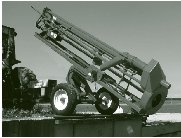
Figure 4.5.2 Example of a pump used to agitate liquid manure prior to application.
