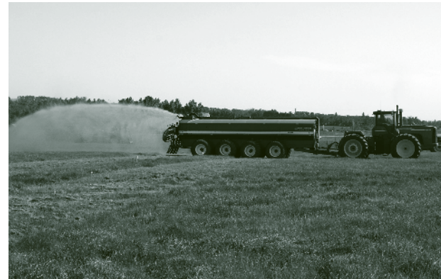
Figure 4.5.1 Examples of Common Liquid Manure Application Equipment
