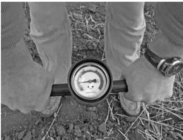
Figure 9. Soil penetrometer used for determining compacted soil horizons.
