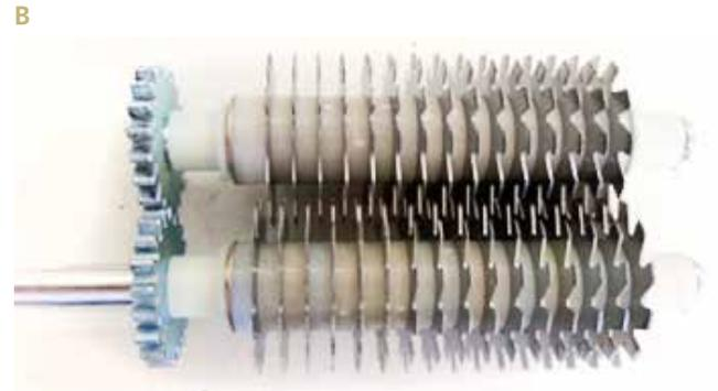
Fig. 1 Mechanical tenderizer (A) and its mechanisms (B) used for making minute steaks.
